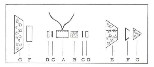
A - Tantalum tube with thermocouple wires spotwelded to side.
